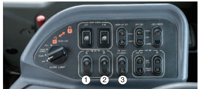
1: Trans. cut-off ON/OFF switch 3: Trans. shifting switch 2: Trans. cut-off set switch
