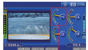
Hybrid system temperature gauge.
