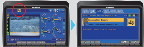
Aftertreatment device regeneration screen
