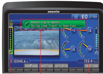
Ecology gauge Ecology guidance Fuel consumption gauge
