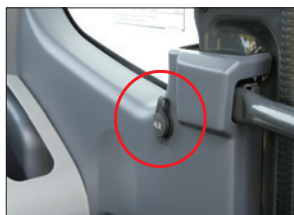
Defroster (conforms to the ISO standard)
