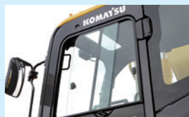
Remote intermittent wiper with windshield washer
