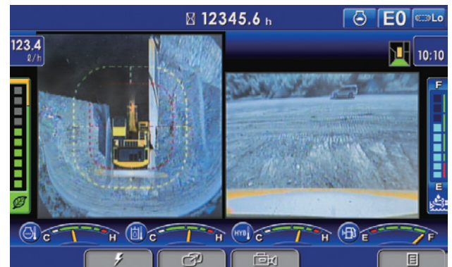
Ecology gauge Ecology guidance Fuel consumption gauge
