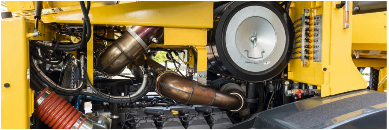
TIER 4 final with dual SCR system.
