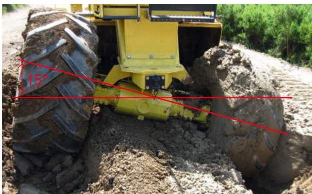
Non-spin oscillating axle +/- 15°.
