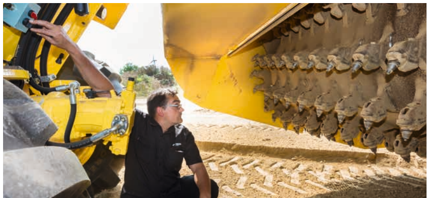
Easy monitoring of the rotor with a safety gap between the control unit and rotor.
