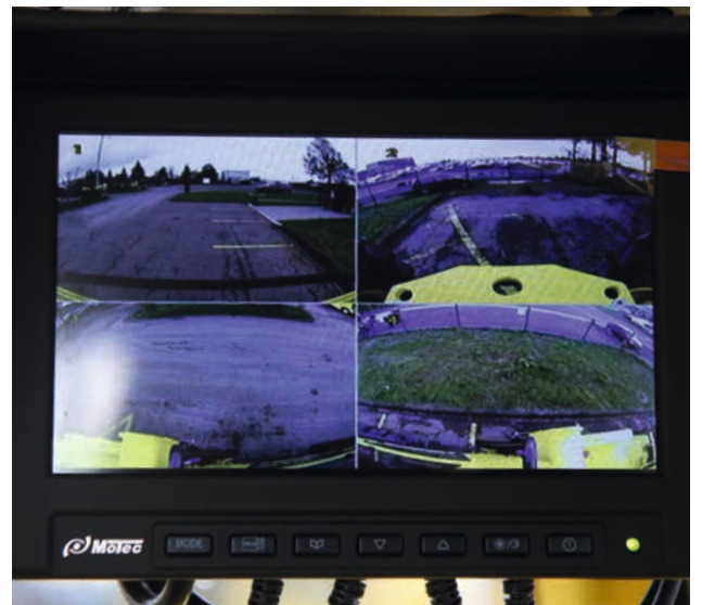
Cameras and a monitor provide the perfect all-round view.
