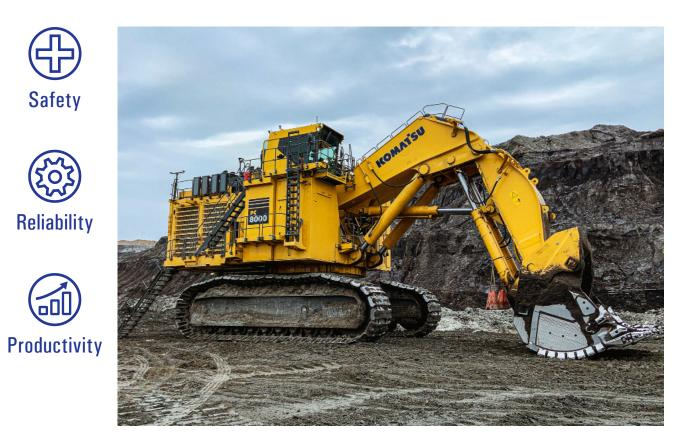
When you need to cycle through large loads, the PC8000 has you covered. It was designed with input from mining operations around the globe to maximize productivity with 240- to 400-ton trucks.
