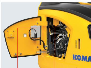
Washer tank Auxiliary hydraulic circuit return filter
