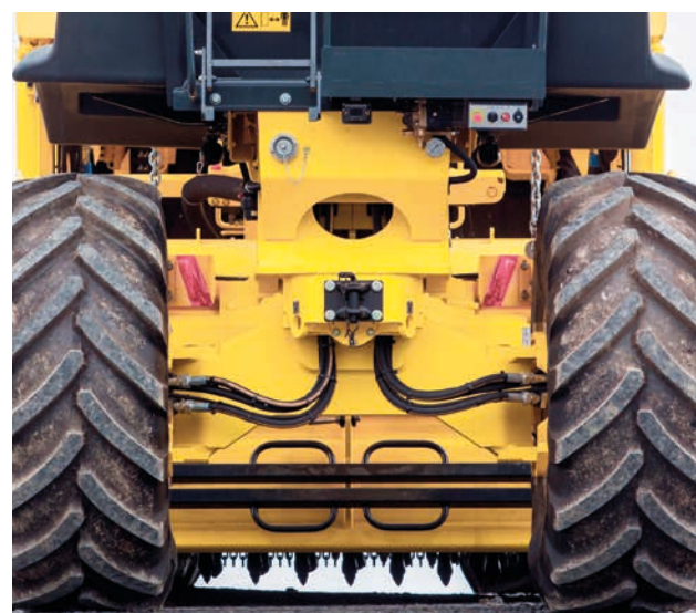
Rear axle with powerful single drives (RS 500).
