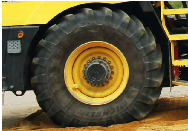
Large wheels for low ground contact pressure.
