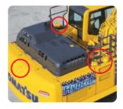
individual camera views of the left, rear and right sides is easily changed using the F4 button. A red line continuously shows where the counterweight will be during swinging and a camera icon indicates which camera is being displayed on individual camera display screen.
