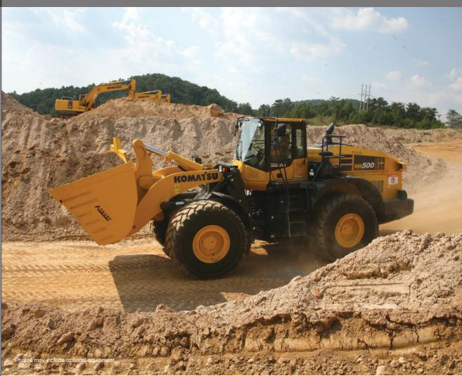
NET HORSEPOWER 353 HP @ 1900 rpm 263 kW @ 1900 rpm **OPERATING WEIGHT** 80,647 – 81,020 lb 36,581 – 36,750 kg **BUCKET CAPACITY** 8.2 – 9.8 yd<sup>3</sup> 6.3 – 7.5 m<sup>3</sup>
