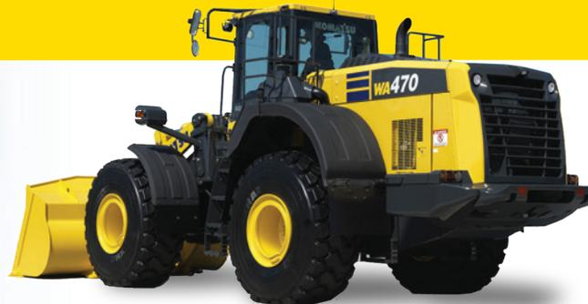
A powerful **Komatsu SAA6D125E-7 engine** provides a net output of 203 kW **272 HP** with 6% improved fuel consumption. This engine is EPA Tier 4 Final emissions certified.
