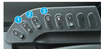
1 Dual mode engine power selection switch
