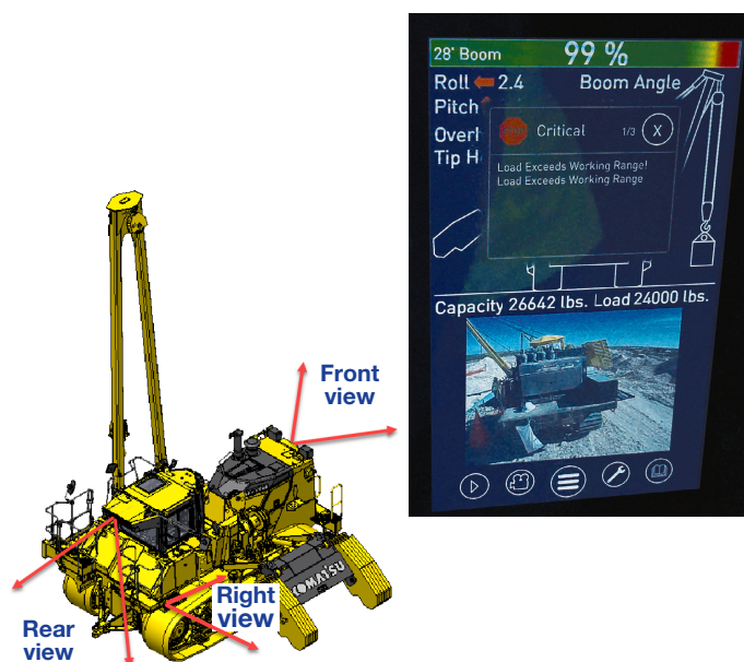
Three cameras provide additional views around the machine. Forward view camera (above), with selectable right-side camera and rearview camera are standard. Load Moment Indicator information is displayed at top of screen.
