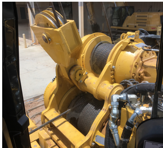
Good view to winch drums for spooling
