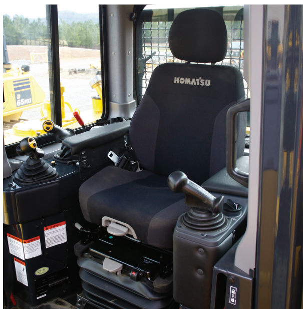
Air-suspension seat with heat is standard
