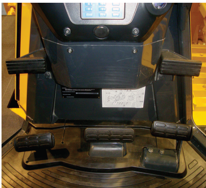
Engine decelerator and brakes can be applied independently
