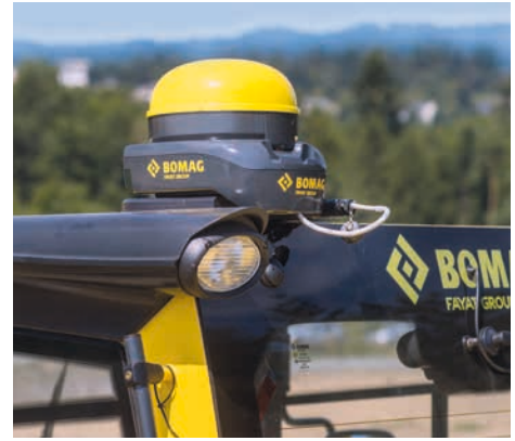
BOMAG StarFire: GPS for accurate mapping and pass counting.
