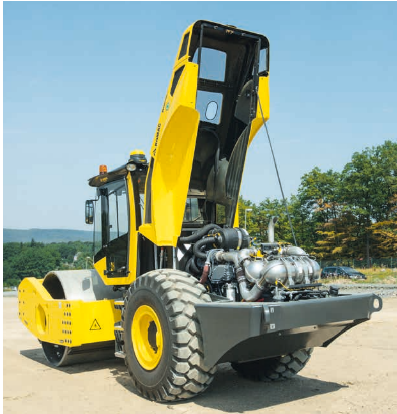
Handy, large, hinged engine hood: all service points are easily accessible.
