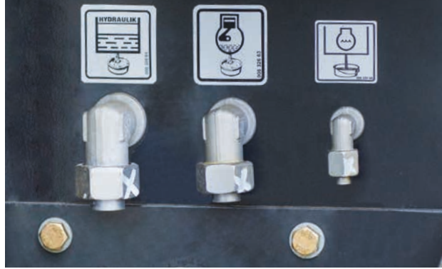
Smart: fluids can be drained externally.
