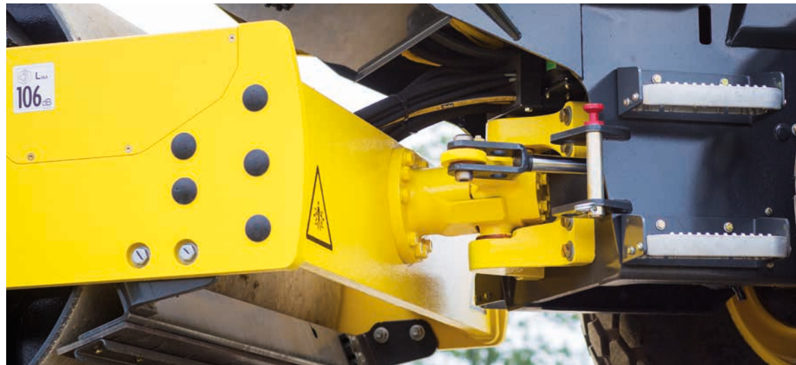
Keep it clean: The articulation joint is maintenance-free; the machine needs no lubrication whatsoever.
