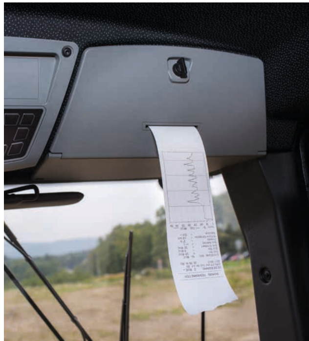
Integrated printer: for documentation of compaction results.
