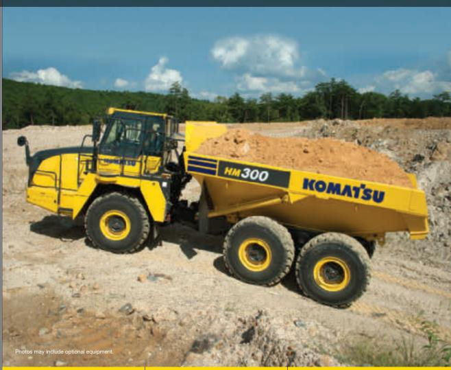
HORSEPOWER Gross: 332 HP 248 kW Net: 324 HP 242 kW PAYLOAD 30.9 US tons 28.0 metric tons **BODY CAPACITY** Heaped (SAE 2:1): 22.4 yd<sup>3</sup> 17.1 m<sup>3</sup>
