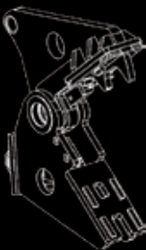
G Jaw Set (Pulverizing) Replaceable Tooth Plate
