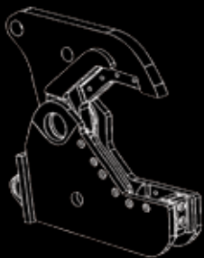
K Jaw Set (Shearing) with Bolt-On Piercing Tips (M-35K ONLY)
