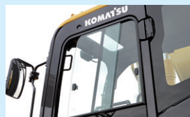
Remote intermittent wiper with windshield washer
