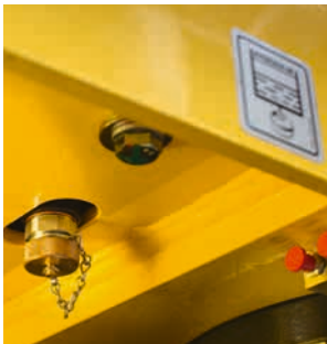
Highly visible markings on service points
