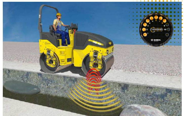
The Economizer measures the material stiffness and indicated the optimal condition
