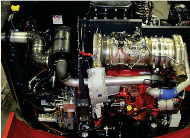
Cummins L9 Series Engine - 338HP with simple Single Module DOC/DPF/SCR unit
