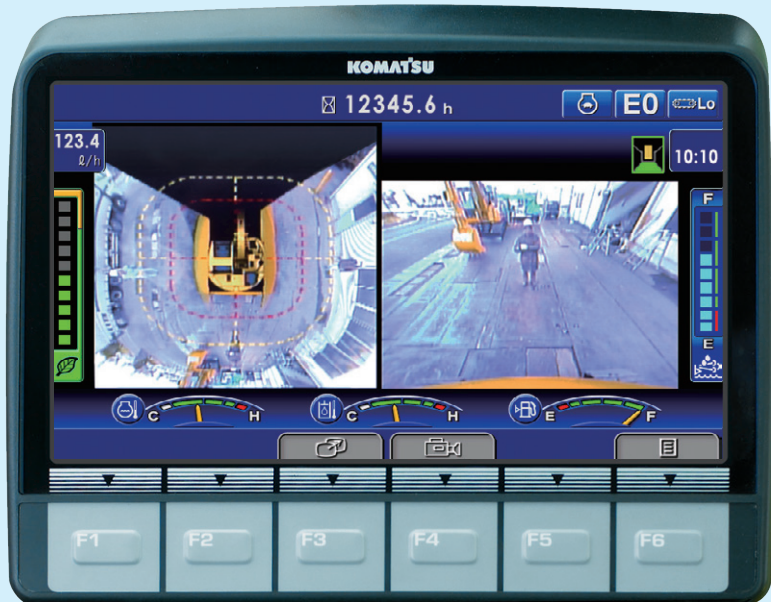
Distance markers are displayed in the monitor to show machine tail swing radius.
